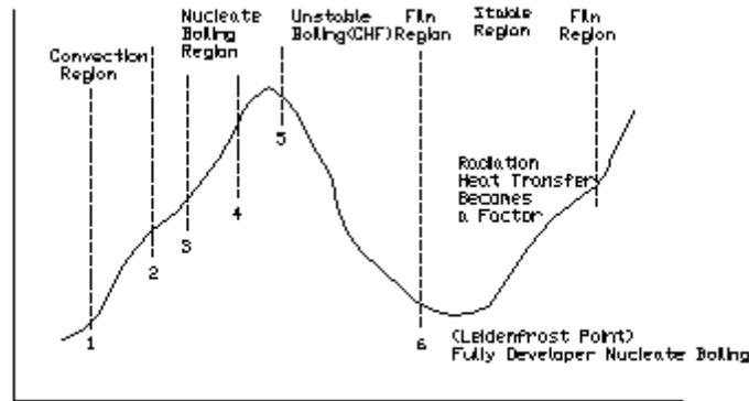
Fig.2 Boiling Curve Showing Regimes of  $\log(t_w - t_s)$  Boiling Heat Transfer.
