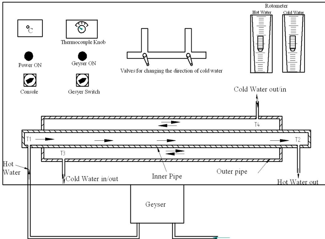
Experimental Setup of Heat Exchanger
