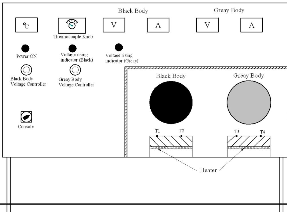
Fig: Line diagram of surface emissivity
