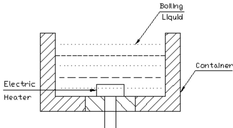
**Fig.1 Pool Boiling with an electric heater for constant energy input.**
