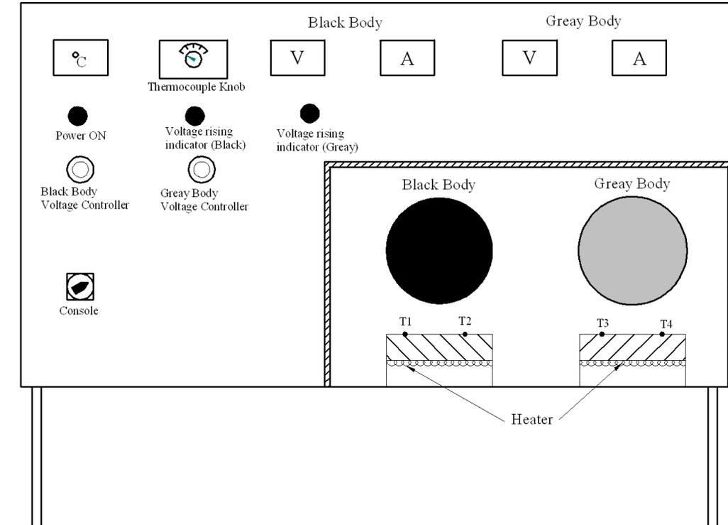
Fig: Line diagram of surface emissivity
